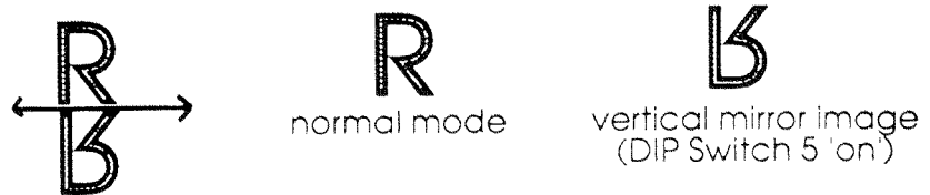
Figure 2.20 Vertical Mirror Image Display
