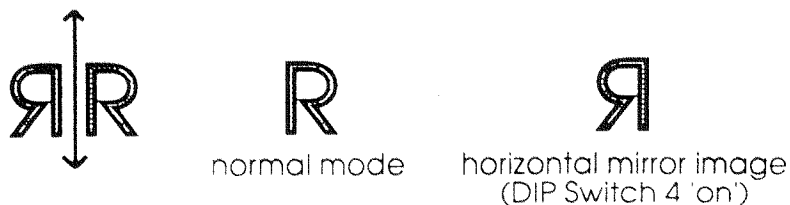
Figure 2.19 Horizontal Mirror Image Display
